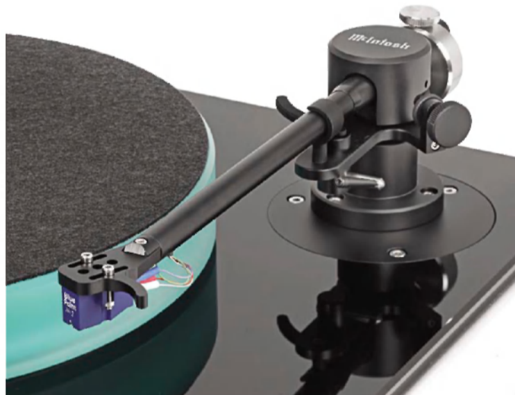
The arm is lowered and lifted with a damped platform, operated by a lever. Manual cueing isn't so easy, because there's little clearance between the flat finger lift and the record surface. Finger lifts are usually curved upward to avoid this difficulty.
