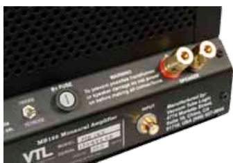
SIMPLICITY APPLIES TO THE SPARSELY POPULATED REAR PANEL: A SINGLE-ENDED RCA PROVIDES SIGNAL CONNECTIVITY, AND A WELL-MACHINED PAIR OF BINDING POSTS FOR SPEAKER CABLES.
